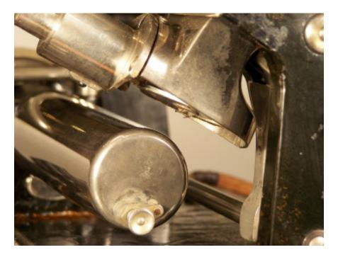
Thomas Macdonald's patented (No.874,973) combination recorder/reproducer. By manipulating a lever above the carriage, the assembly can be simultaneously moved slightly to the rear and the cutting stylus gently lowered into recording position. Moving the lever in the opposite direction will shift the assembly slightly toward the front and gently lower the playing stylus into position.
